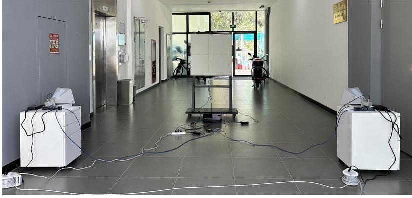
Fig. 2. Field test with an IRS prototype that consists of 400 REs and provides 4 phase shift options  $\{0, \pi/2, \pi, 3\pi/2\}$  on each RE.
