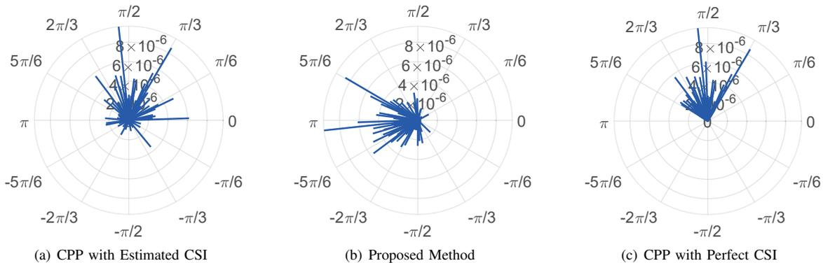
Fig. 4. Plots of the optimized reflected channels  $h_n e^{j\theta_n}$  by the different methods when  $N = 100$  and  $K = 4$ .
