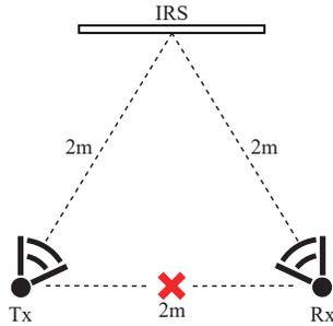
Fig. 3. Layout drawing of the testbed. The transmit and receive antennas are oriented such that the direct propagation is nullified.
